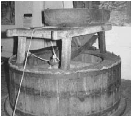
A vat to cover the mill stone.
